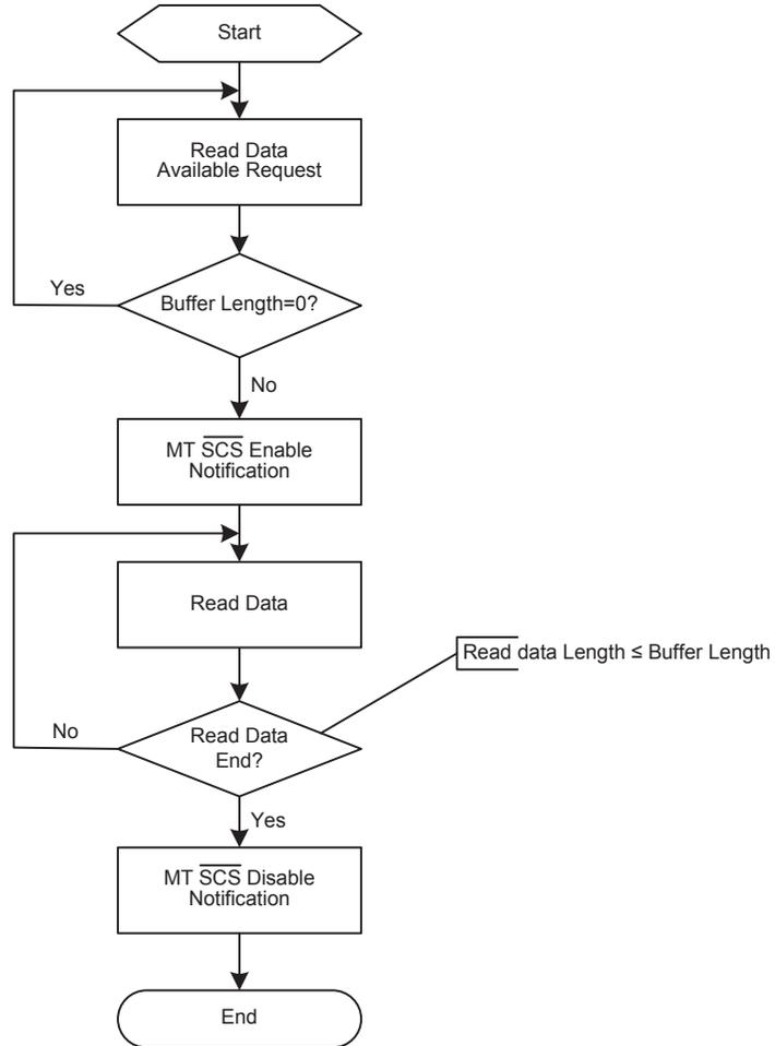
**Master Transmitter  $\overline{\text{SCS}}$  Enable/Disable Notification**
