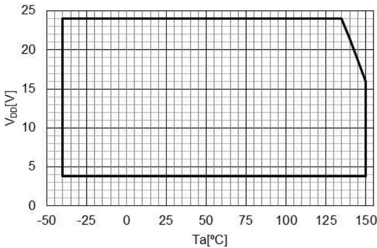
Figure 3. Supply Voltage
