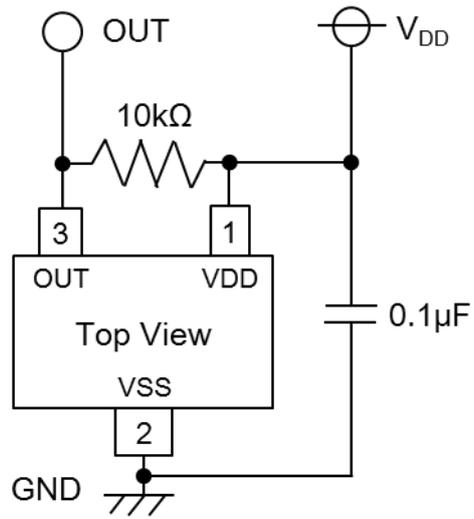
Figure 8. Recommended External Circuit
