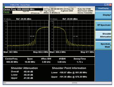
Figure 5. DTMB (CTTB) shoulder attenuation
