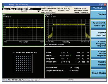
Figure 3. DTMB (CTTB) IQ quad view
