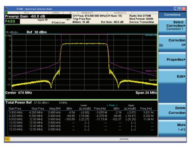
Figure 6. DTMB (CTTB) spectrum emission mask
