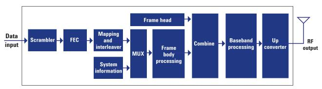
Figure 1. Block diagram of DTMB (CTTB) system
