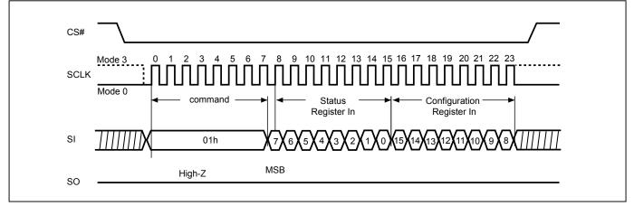
Note : The CS# must go high exactly at 8 bits or 16 bits data boundary to completed the write register command.
