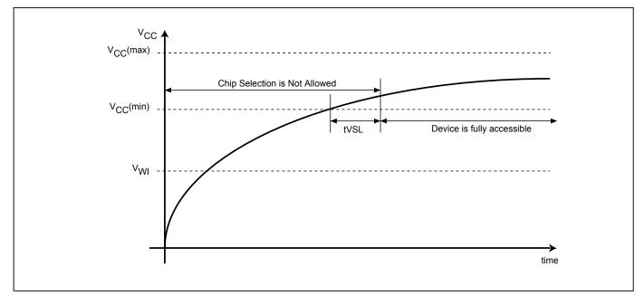
Note: VCC (max.) is 2.0V and VCC (min.) is 1.65V.
