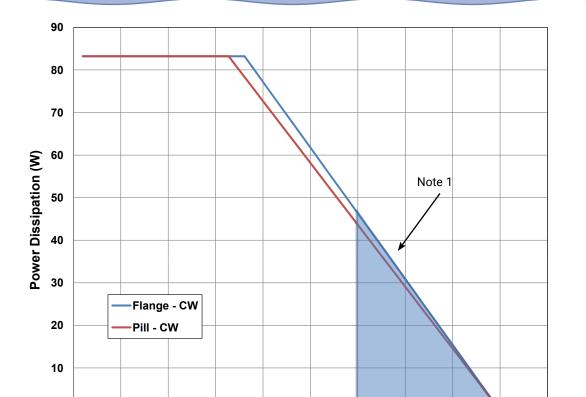
Figure 5. - Transient Power Dissipation De-Rating Curve
