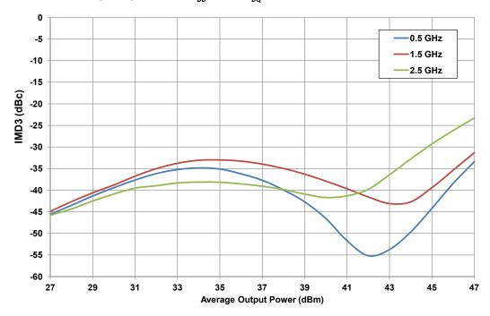
Figure 4. - Third Order Intermodulation Distortion vs Frequency measured in Broadband Amplifier Circuit CGHV40100-AMP Spacing = 1 MHz,  $V_{DD}$  = 50 V,  $I_{DO}$  = 600 mA, Tcase = 25°C
