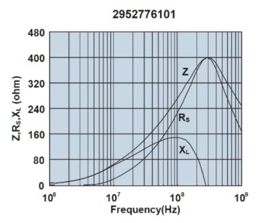
Impedance, reactance, and resistance vs. frequency.
