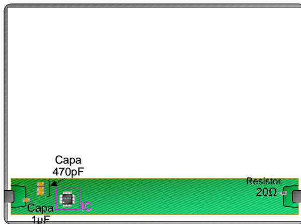
Figure 41. Layout example for ESD protection
