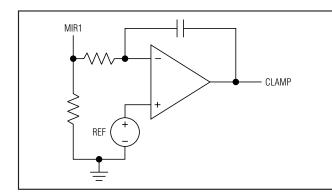
Figure 1. Current Clamp from Current Feedback
