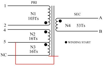
Core is connected to Pin 5 by naked wire
