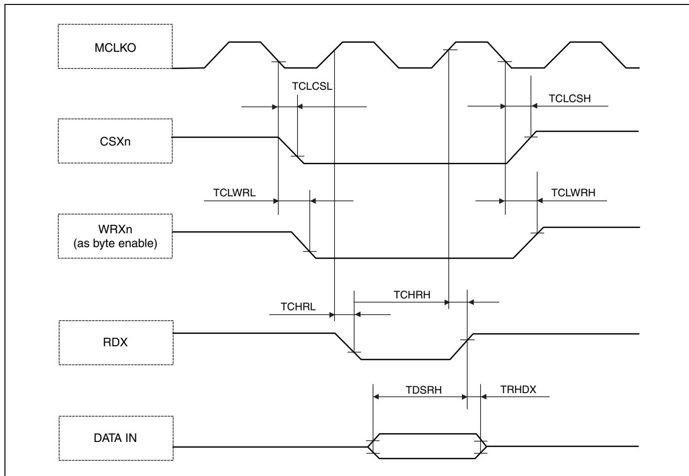
*Synchronous write access - byte control type*
