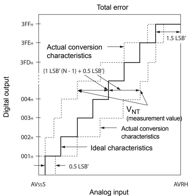
$$1\text{LSB}' (\text{ideal value}) = \frac{\text{AVRH} - \text{AV}_{\text{SS}5}}{1024} [\text{V}]$$
