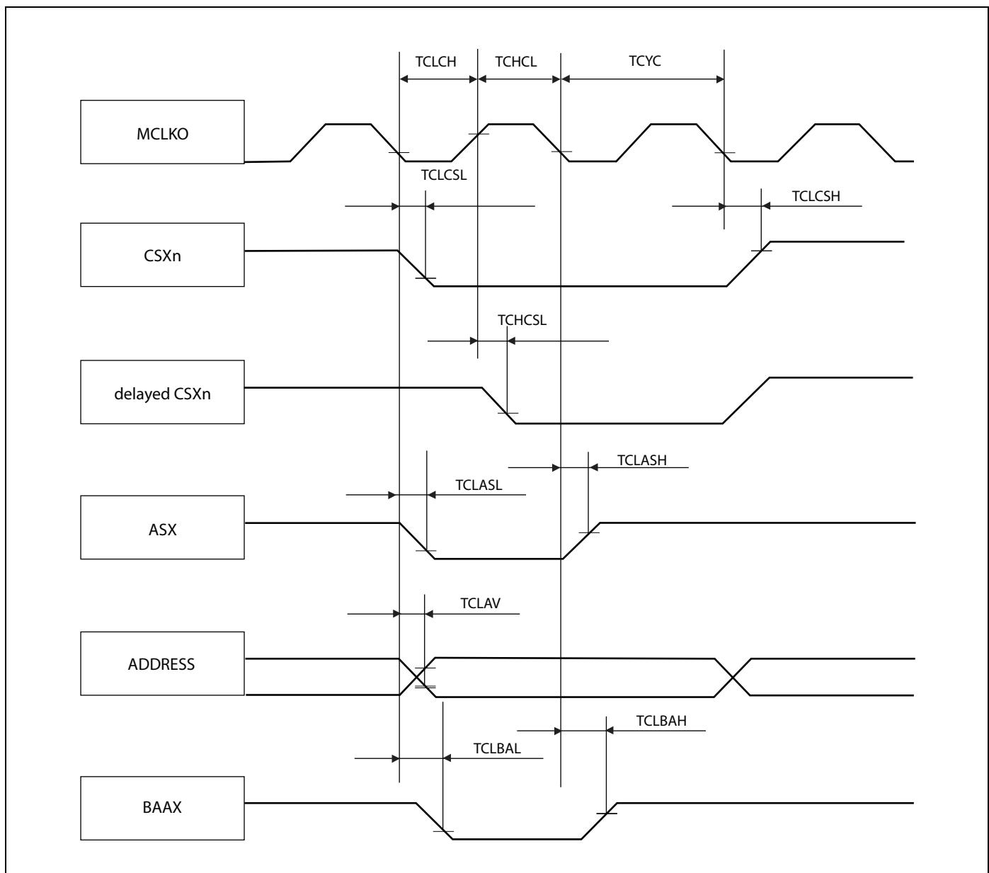
*Synchronous/Asynchronous read access with external MCLKI input*
