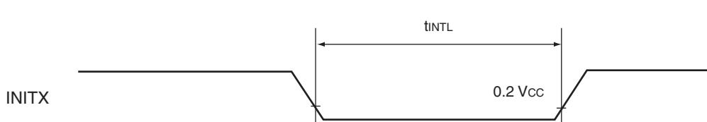
**15.7.3 LIN-USART Timings at  $V_{DD5} = 3.0$  to  $5.5$  V**
