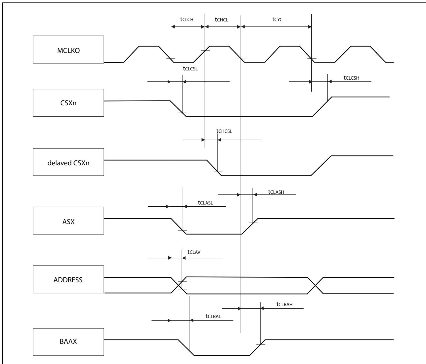
*Synchronous/Asynchronous read access with external MCLKI input*
