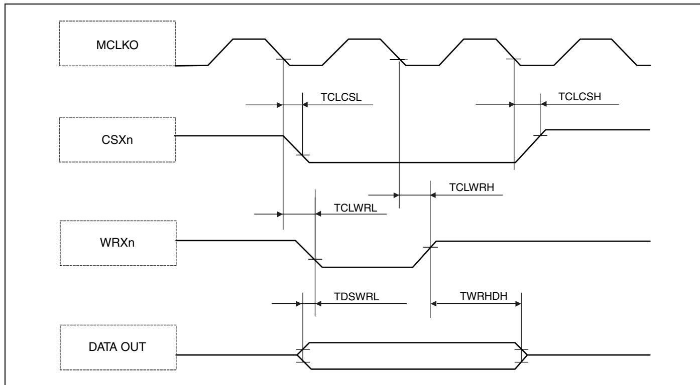
**Asynchronous write access - byte control type**
