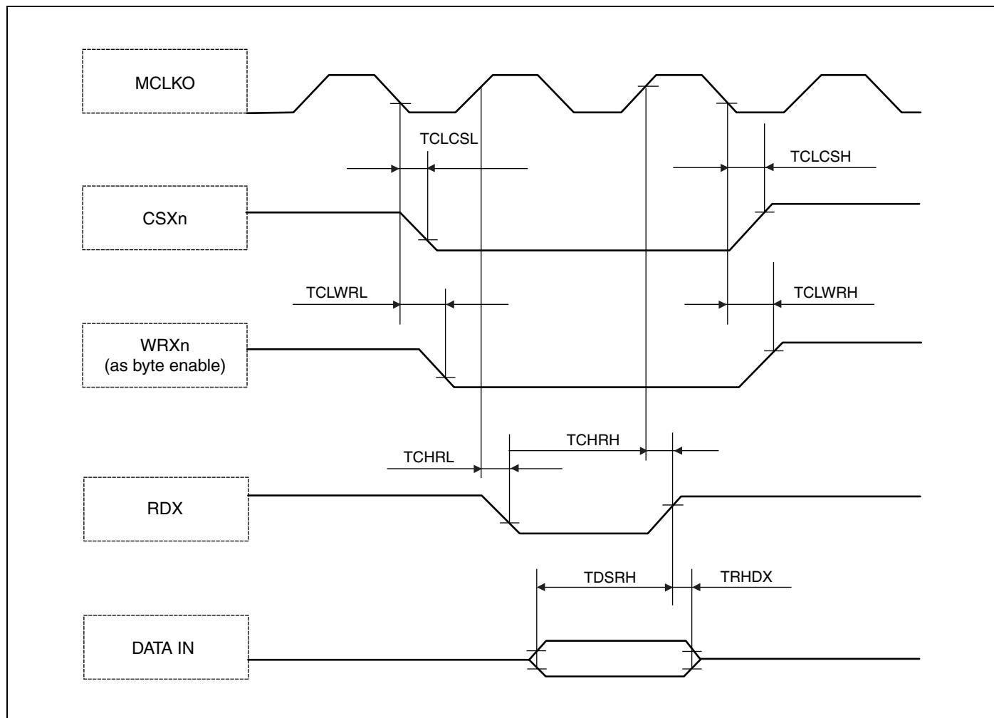
*Synchronous write access - byte control type*
