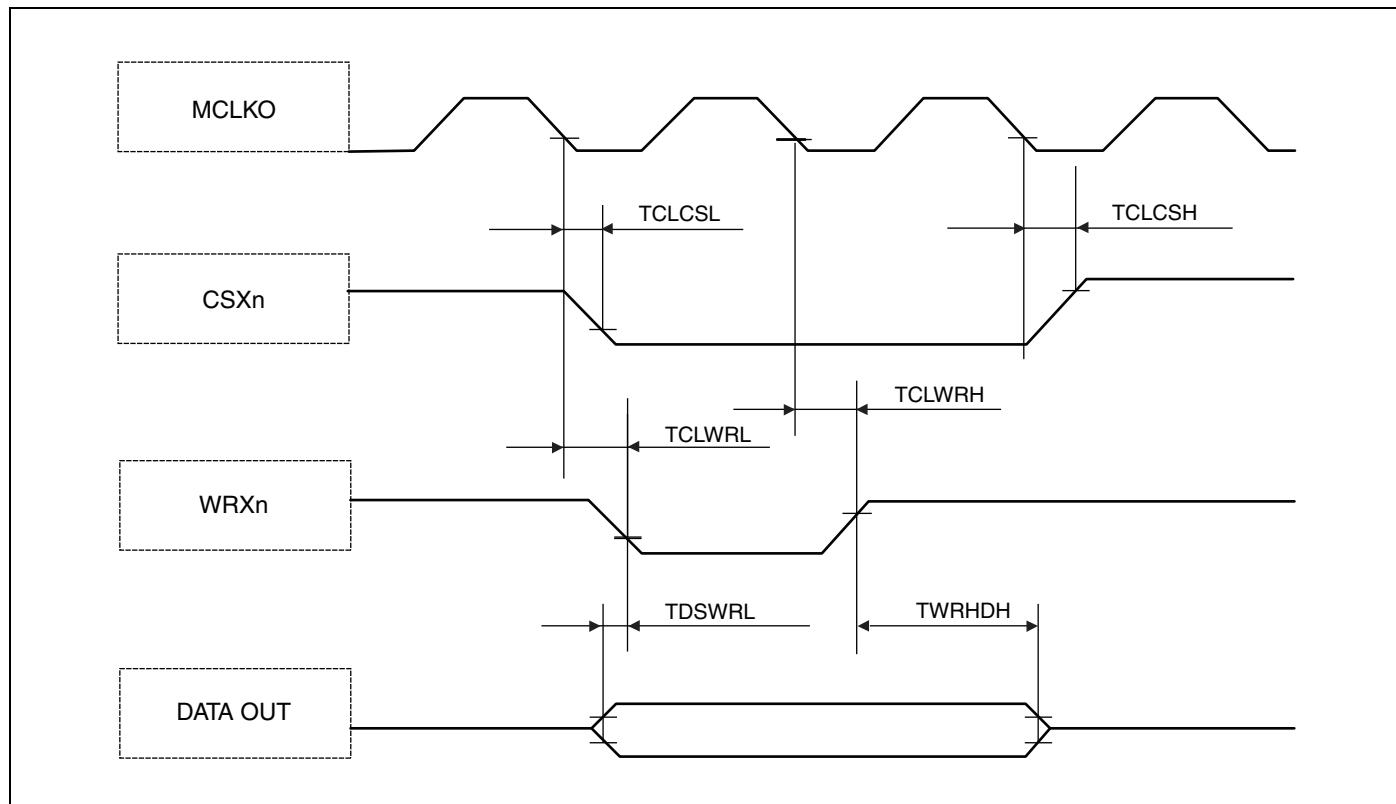
**Asynchronous write access - byte control type**
