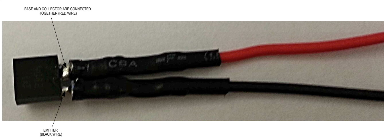
Figure 3. 2N3906 Diode-Connected Transistor Assembly (Not Included)
