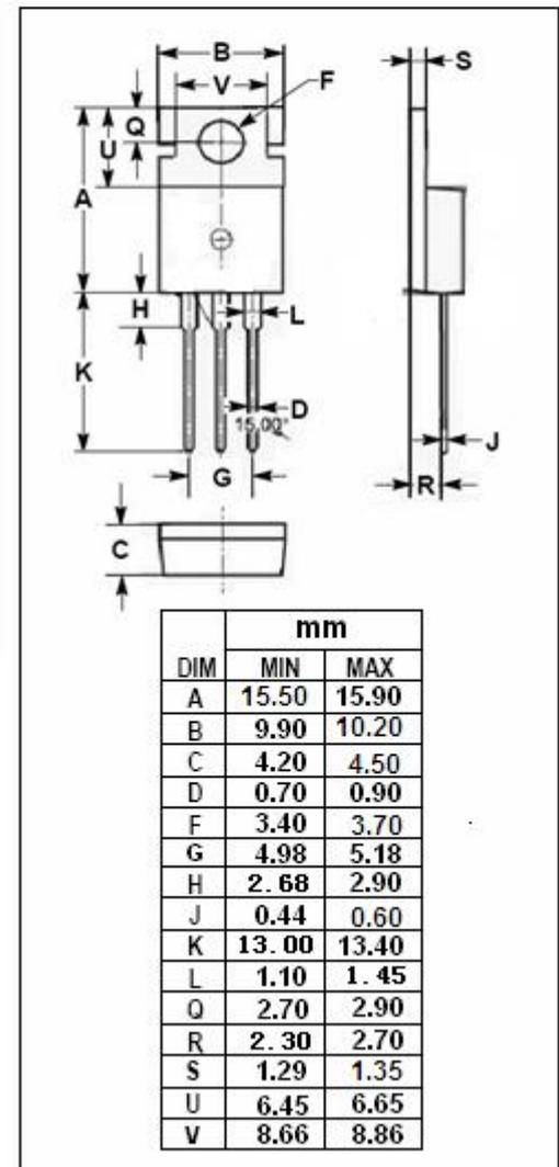
**Isc N-Channel MOSFET Transistor**
