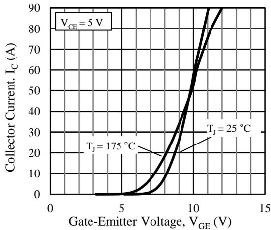
Figure 10. Transfer Characteristics
