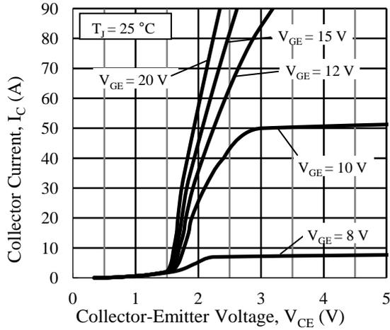
Figure 8. Output Characteristics ( $T_J = 25\text{ }^\circ\text{C}$ )
