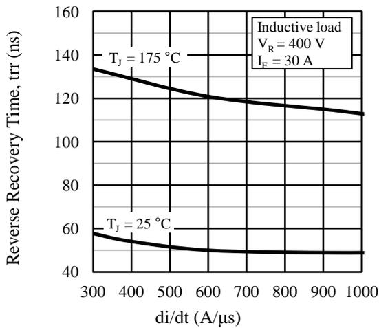
Figure 24. Diode Reverse Recovery Time vs. di/dt
