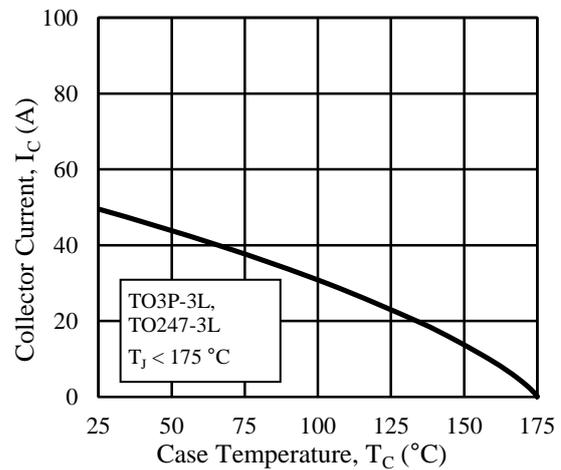
Figure 5. Collector Current vs. TO3P and TO247 Case Temperature
