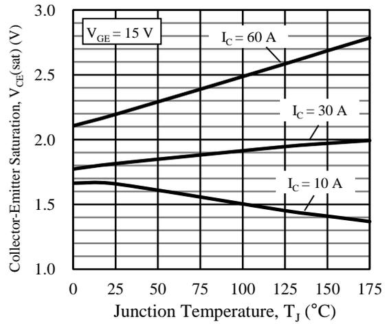
Figure 11. Saturation Voltage vs. Junction Temperature
