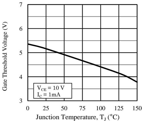
Figure 12. Gate Threshold Voltage vs. Junction Temperature
