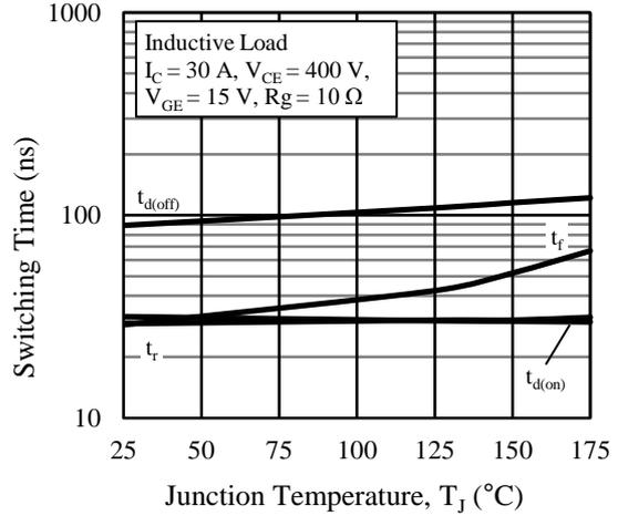
Figure 15. Switching time vs. Junction Temperature
