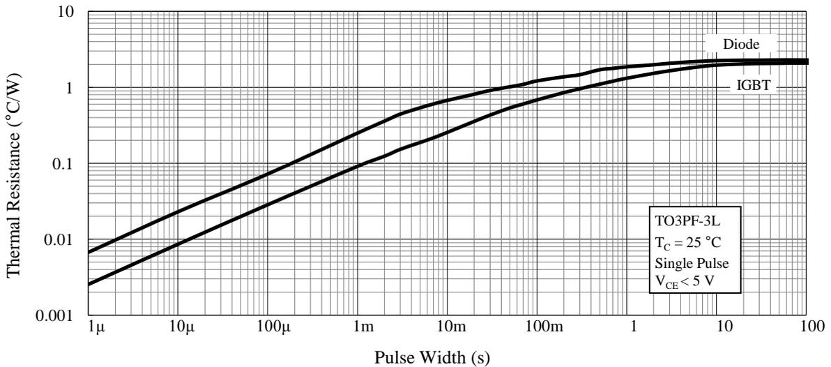
Figure 28. Transient Thermal Resistance (TO3PF-3L)
