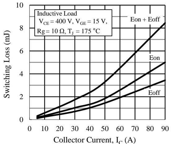
Figure 19. Switching Loss vs. Collector Current
