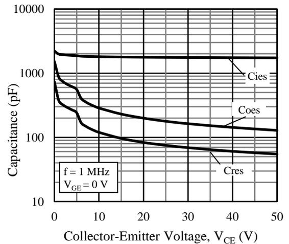
Figure 13. Capacitance Characteristics
