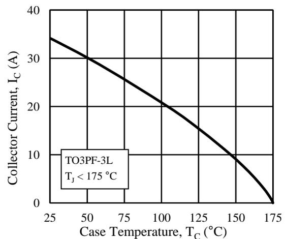
Figure 7. Collector Current vs. TO3PF Case Temperature
