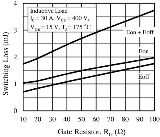
Figure 20. Switching Loss vs. Gate Resistor
