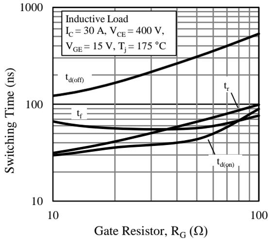
Figure 17. Switching Time vs. Gate Resistor
