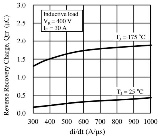
Figure 25. Diode Reverse Recovery Charge vs. di/dt
