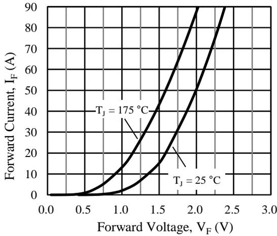
Figure 22. Diode Forward Characteristics
