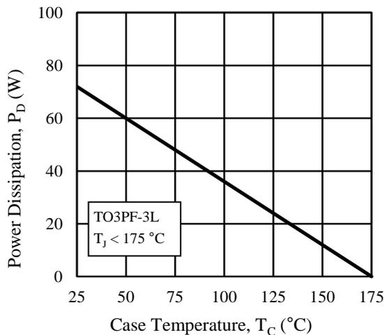
Figure 6. Power Dissipation vs. TO3PF Case Temperature
