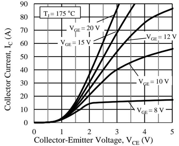
Figure 9. Output Characteristics ( $T_J = 175\text{ }^\circ\text{C}$ )
