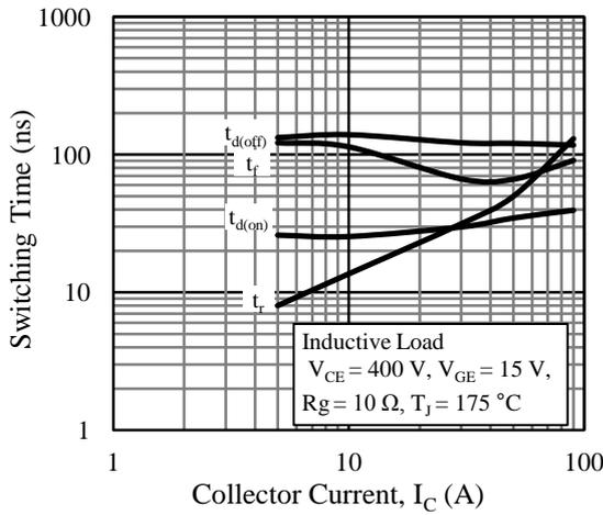
Figure 16. Switching Time vs. Collector Current
