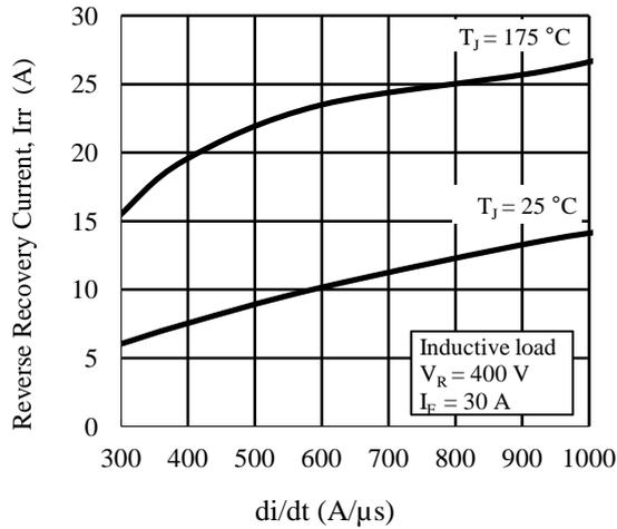
Figure 26. Diode Reverse Recovery Current vs. di/dt
