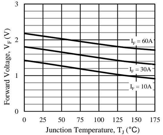
Figure 23. Diode Forward Voltage vs. Junction Temperature
