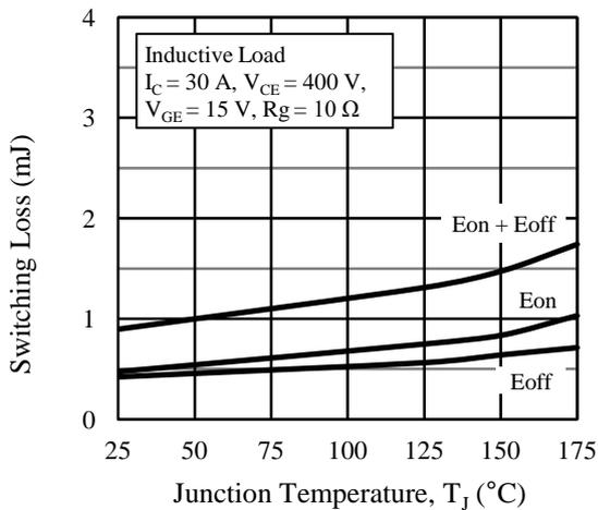
Figure 18. Switching Loss vs. Junction Temperature
