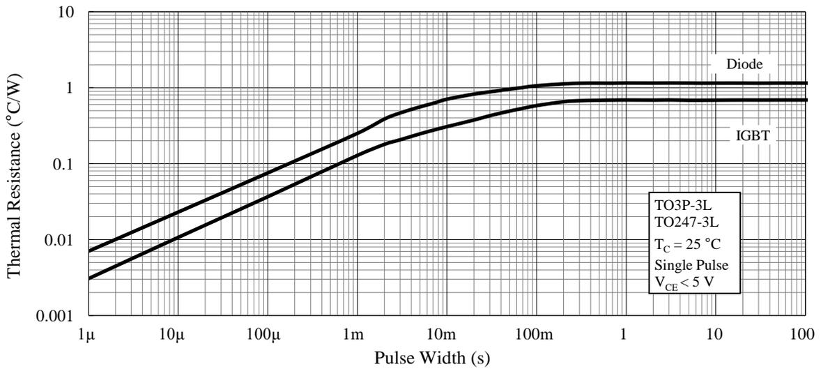
Figure 27. Transient Thermal Resistance (TO3P-3L and TO247-3L)
