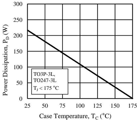
Figure 4. Power Dissipation vs. TO3P and TO247 Case Temperature
