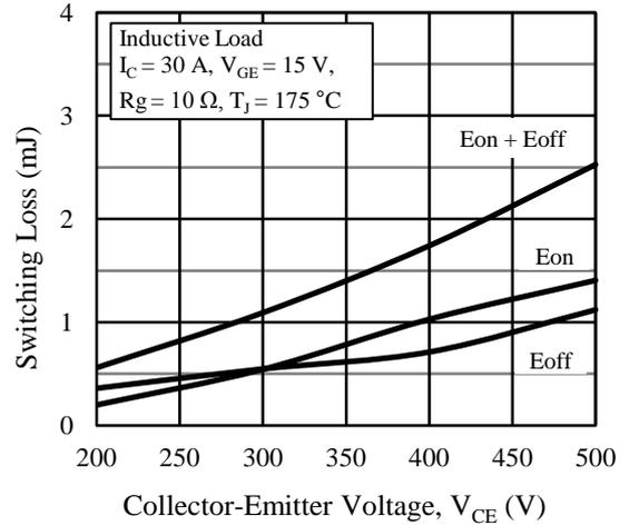
Figure 21. Switching Loss vs. Collector-Emitter Voltage
