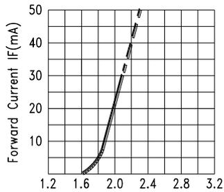
Forward Voltage Vf (V)
