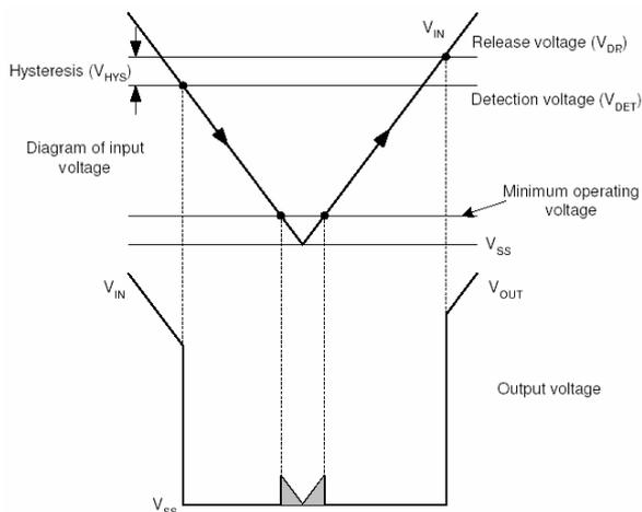
Note: For voltage  $V_{IN}$  less than minimum operating voltage (shaded region on the diagram), voltage of output terminal is undefined for CMOS output product.
