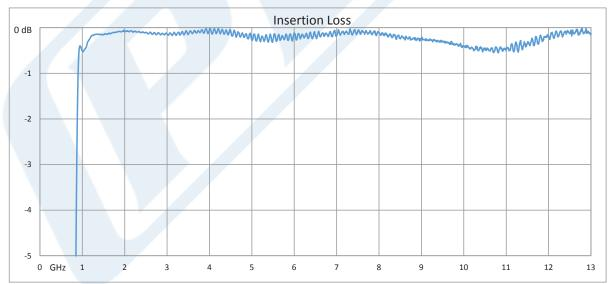
Click the following link (or enter part number in "SEARCH" on website) to obtain additional part information including price, inventory and certifications: 7 Section Highpass Filter With SMA Female Connectors Operating From 1 GHz to 13 GHz PE87FL1018
