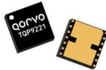
14 Pin 7x7 mm leadless SMT Package
