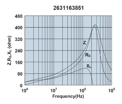
Impedance, reactance, and resistance vs. frequency.
