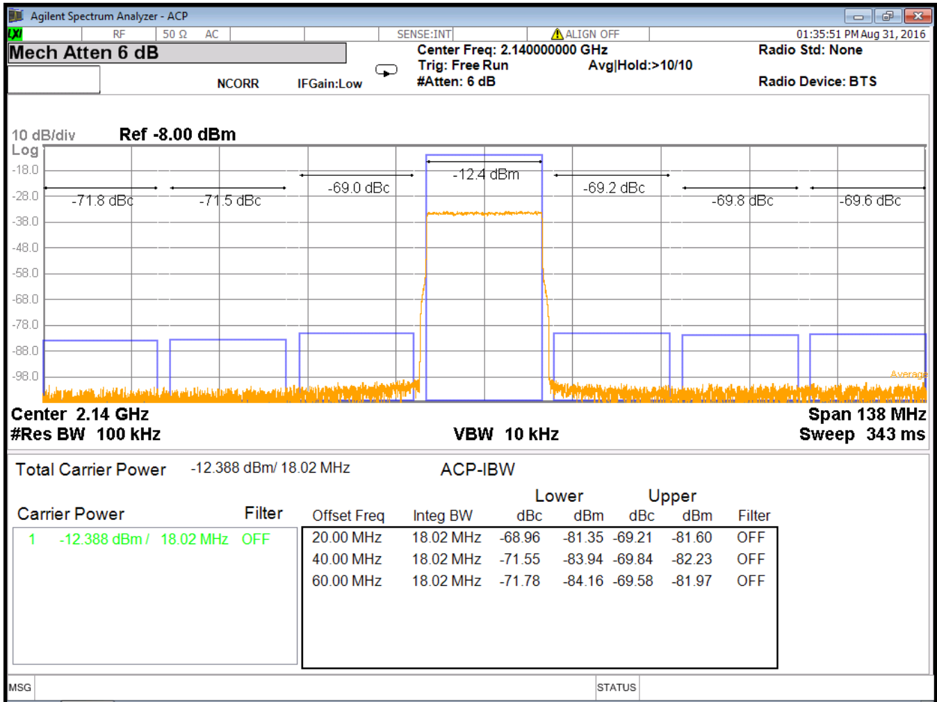
Figure 145. Dual band ACPR Performance in Downlink Band 1 with On-chip PLL
