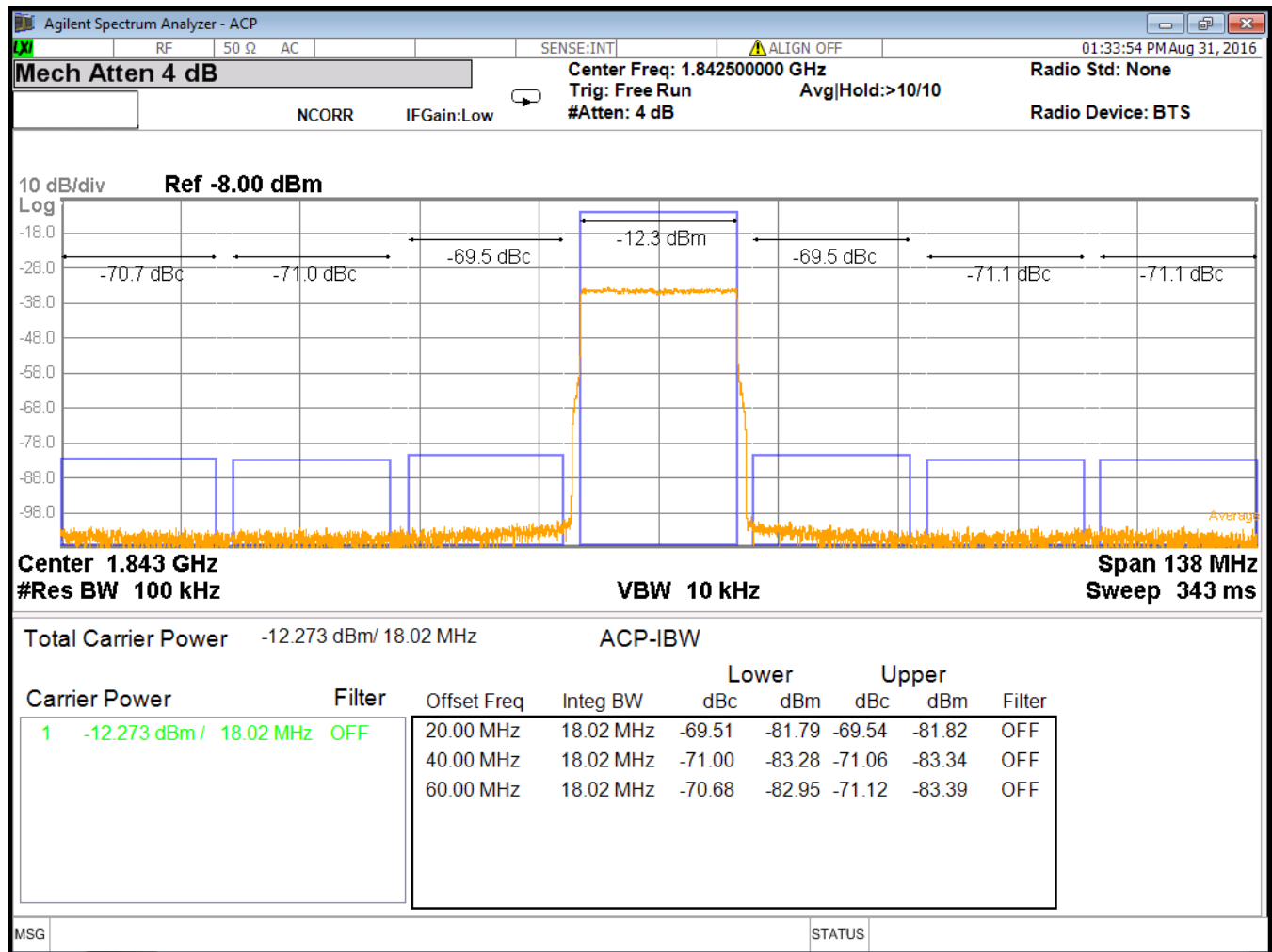
Figure 144. Dual band ACPR Performance in Downlink Band 3 with On-chip PLL
