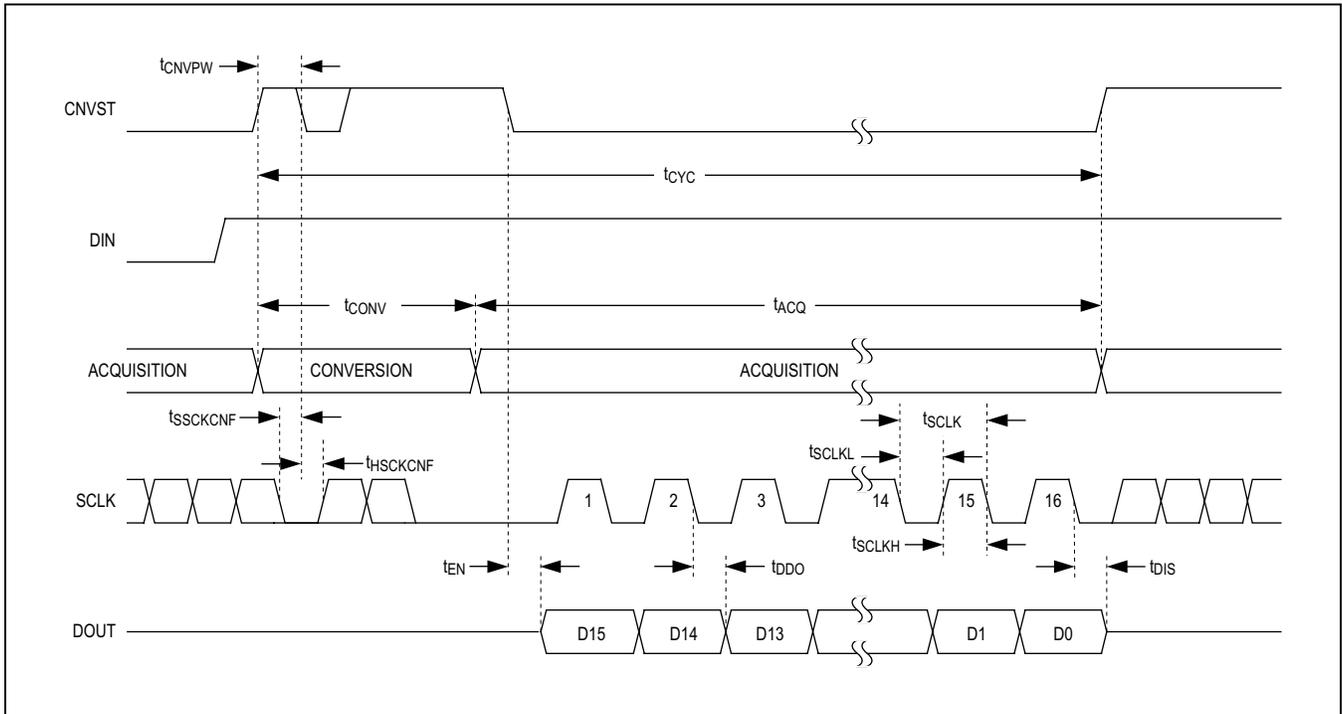
Figure 7. CS No Busy Indicator Mode Timing
