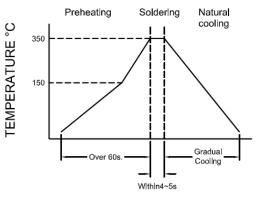
Iron Soldering times: 1 times max
