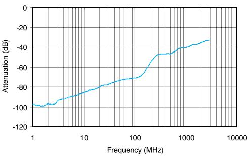
Figure 3. Crosstalk vs Frequency
