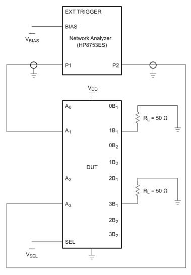
Figure 7. Test Circuit for Crosstalk (X<sub>TALK</sub>)
