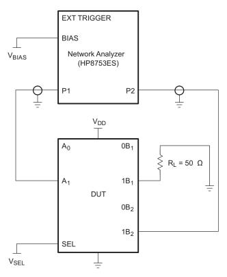
Figure 8. Test Circuit for Off Isolation (O<sub>IRR</sub>)
