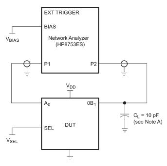
Figure 6. Test Circuit for Frequency Response (BW)
