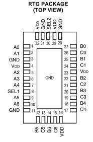
The exposed center pad must be connected to GND.
