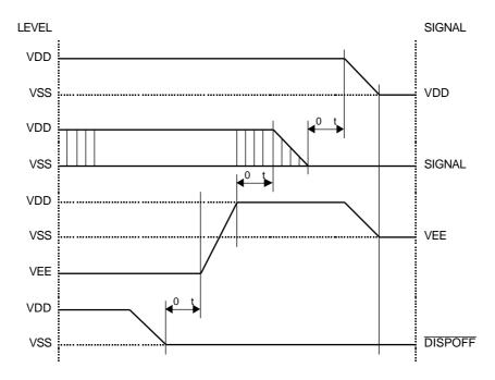
Please maintain the above sequence when turning on and off the power supply of the module. If DISPOFF is supplied to the module while alternate signal for LCD driving (M) is unstable, DC component will be supplied to the LCD panel. This may cause damage the LCD module.
