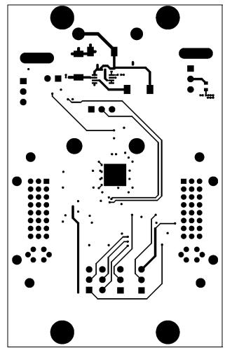
Figure 6. MAX3815 EV Kit PC Board Layout—Solder Side
