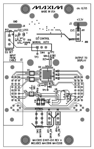
Figure 2. MAX3815 EV Kit PC Component Placement Guide—Component Side
