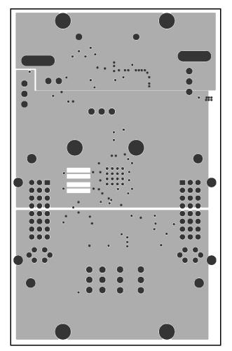
Figure 5. MAX3815 EV Kit PC Board Layout—Power Plane
