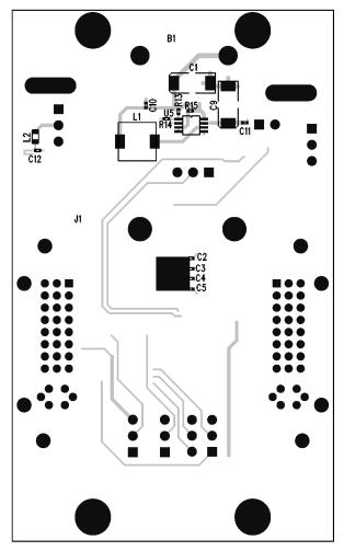
Figure 7. MAX3815 EV Kit PC Component Placement Guide—Solder Side
