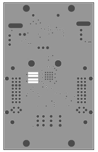
Figure 4. MAX3815 EV Kit PC Board Layout—Ground Plane
