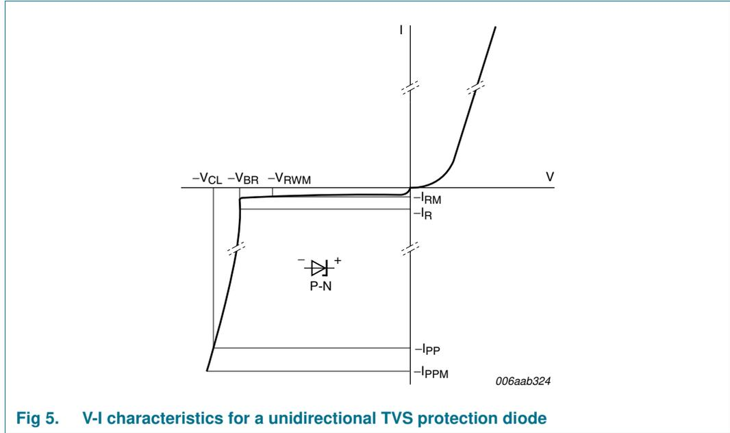
**Fig 5. V-I characteristics for a unidirectional TVS protection diode**
